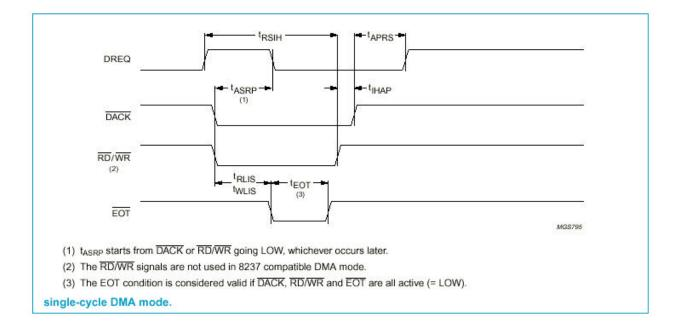
The timing diagram of SH7709 specifies tDRQS = 12 ns (DREQ setup time) and tDRQH = 8 ns (DREQ hold time) relative to a falling edge of CKIO. If the DRQ signal generated by the ISP1181 does not meet the tDRQS timing in the current bus cycle, it will be sensed on the next falling edge of CKIO, and the DACK will be generated accordingly.
